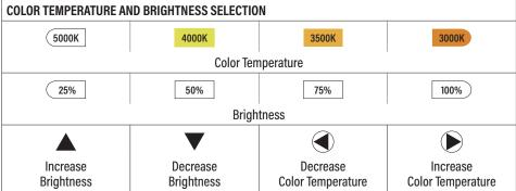
Power the light off then power it on, the last saved brightness (which is saved by the button "SAVE") and the last saved color temperature (which is saved by the button "SAVE" or "OFF") will be displayed by default. The defaulted factory setting of the light is 100% brightness and 4000K.
