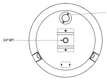
Note: Must remove and disconnect top mount sensor socket before bracket installation (if pre-installed) and replace with cover plate and gasket.
