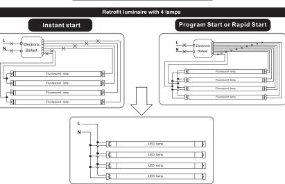
$\triangle$  The below ballast wiring represents typical configuration. The actual ballast wiring varies according to ballast model. It is not needed to change socket (if in good condition) to operate double ended lamps, regardless the type of sockets. Please make sure one side of fixture is connected to Live (L) and the other side to Neutral (N).
